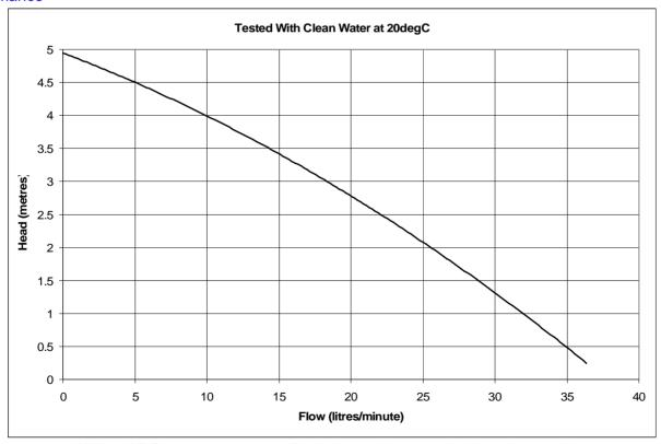
VM and DC pumps are not self-priming and are not designed to run dry. The company reserves the right change specifications.
