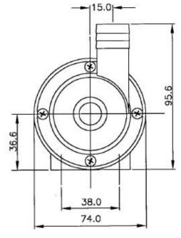
mounting foot fixing holes:M5
