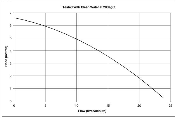
DC pumps are not self -priming and are not designed to run dry. The company reserves the right change specifications.
