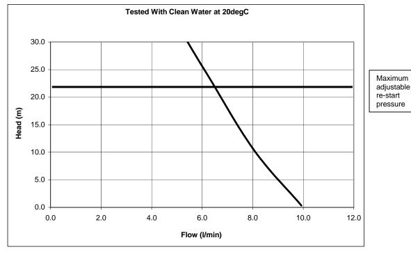
NOTE: These diaphragm pumps are designed for use with clean fluids. Solids will cause reduced performance and damage the pump.
